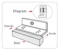
Step 9: Fix Z- bracket to relevant position on the door leaf. (Note: Keep tight contact between the armature plate and the lock)
