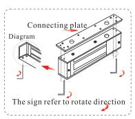
Step 3: Use Allen key to separate the connecting plate from the bottom of the lock. Be careful to hold the screw to prevent slipping.
