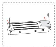
Step 2: Use cross screwdriver to dismount the anti-dismantle screw on the lock.
