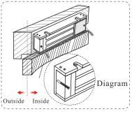
Step 5: Use cross screwdriver to fix the anti-dismantle screw onto the lock.
