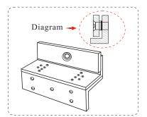
Step 8: Install the armature plate to the Z- bracket (See schematic diagram in Fig.8).
